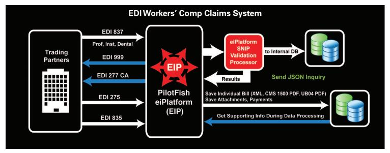
A batch workflow showing EDI 837 from a Trading Partner, ingested and traversing through the PilotFish SNIP Validation Processor then into an Internal DB which generates an EDI 999 and an EDI 277. The EDI 275 and EDI 835 from the Trading Partner's Source System is ingested by PilotFish as an individual bill with saved attachments and payments then transported as a JSON inquiry to the database which yields supporting info during data processing.
